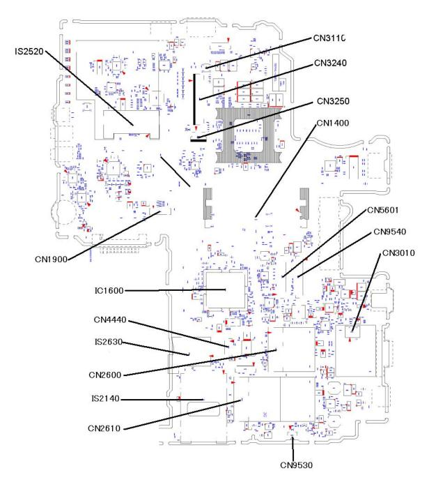
Figure B-1 System board(FW3SY\*) layout (front)
